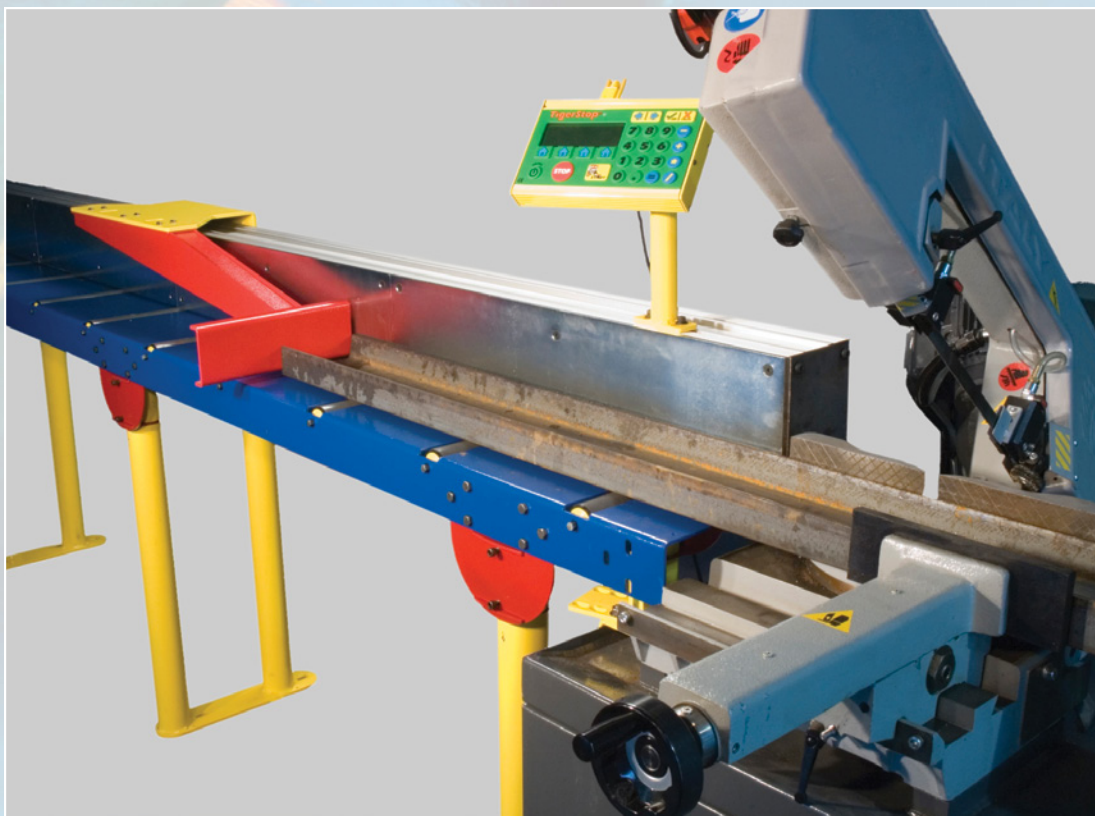
The TT connected with the SIK Switch is push feeding the material from left to right.
